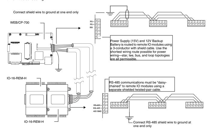
Fig. 11. Power and RS-485 cabling between WEB/CP-700 and remote I/O modules
